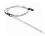
AUTOaccurate-sensor For Hei-VAP Expert Control and Hei-VAP Ultimate Control. Only in combination with glassware set G3, G3 XL or G6 P/N 569-00040-00
