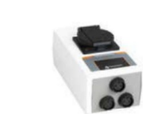
Switchbox Connect up to three rotary evaporators to one vacuum pump If no vacuum is required or when the required vacuum has been reached, the pump is switched off automatically. Prevents excess energy consumption. For applications with different pressure settings, each evaporator must be equipped with vacuum valve and non-return valve. Delivery includes three non-return valves. Suitable only for Hei-VAP Control models Weight 0.6 kg, w/d/h 80×45×160 mm P/N 569-00400-00
